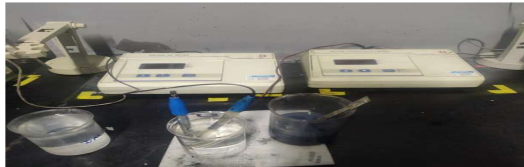
pH meter and conductivity meter Function : To check the pH and conductivity of the different baths
