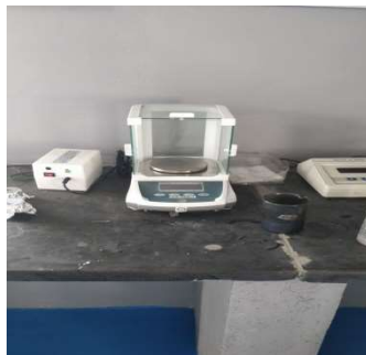
Weigh Balance Function : weight of CED sample during NVM testing
