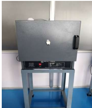
MUFFLE FURNACE Function: Ash content in CED bath
