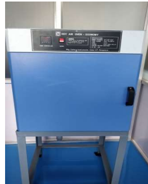
Hot air oven Function: NVM in CED bath Oil content test
